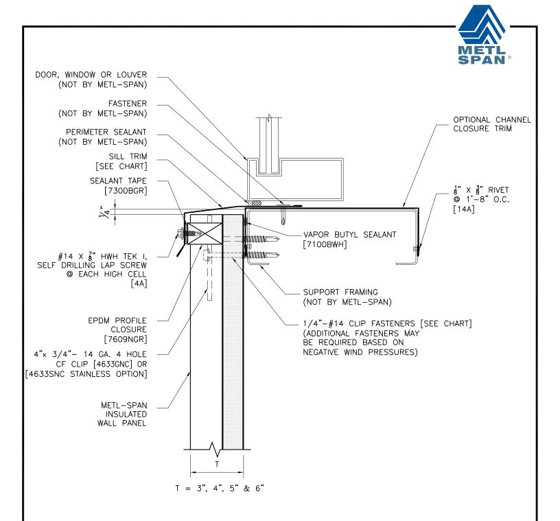
REFER TO SHEET "CI-INFO" FOR ADDITIONAL INFORMATION REGARDING THE APPLICATION OF SEALANTS, FASTENERS, AND CLOSURE MATERIALS. CONSULT METL-SPAN TO DETERMINE ALLOWABLE LOAD AND SPACING OF ATTACHMENT FASTENERS.
