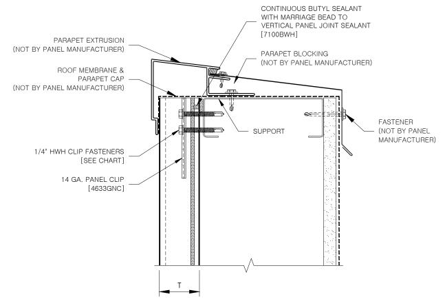
REFER TO SHEET "CI-CF-INFO" FOR ADDITIONAL INFORMATION REGARDING THE APPLICATION OF SEALANTS, FASTENERS, AND CLOSURE MATERIALS. CONSULT METL-SPAN TO DETERMINE ALLOWABLE LOAD AND SPACING OF ATTACHMENT FASTENERS.
