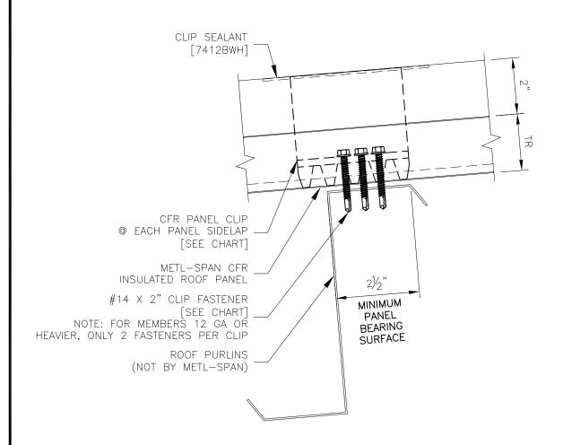
REFER TO SHEET "CI-INFO" FOR ADDITIONAL INFORMATION REGARDING THE APPLICATION OF SEALANTS, FASTENERS, AND CLOSURE MATERIALS. CONSULT METL-SPAN TO DETERMINE ALLOWABLE LOAD AND SPACING OF ATTACHMENT FASTENERS.
