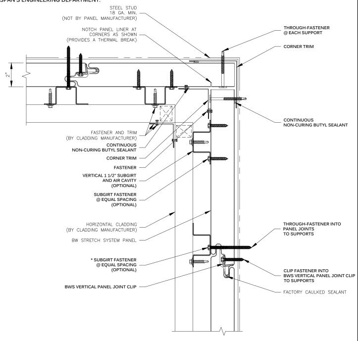
VERTICAL PANEL JOINT CLIP INSIDE CORNER - w/ VERTICAL SUBGIRT BW STRETCH SYSTEM<sup>TM</sup>
