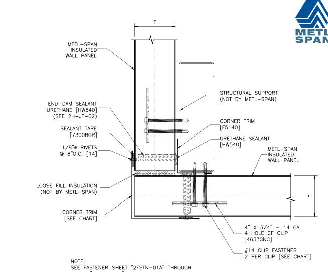
NOTE: SEE FASTENER SHEET "2FSTN-01A" THROUGH SHEET "2FSTN-01D" FOR FASTENING APPLICATION. ADDITIONAL INTERIOR FASTENERS MAY BE REQUIRED BASED ON NEGATIVE WIND PRESSURES.
