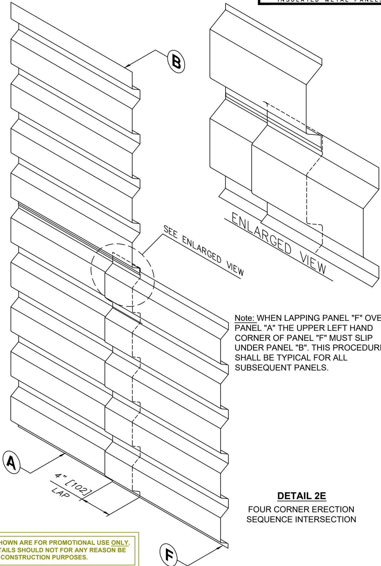
Note: WHEN LAPPING PANEL "F" OVER PANEL "A" THE UPPER LEFT HAND CORNER OF PANEL "F" MUST SLIP UNDER PANEL "B". THIS PROCEDURE SHALL BE TYPICAL FOR ALL SUBSEQUENT PANELS.
