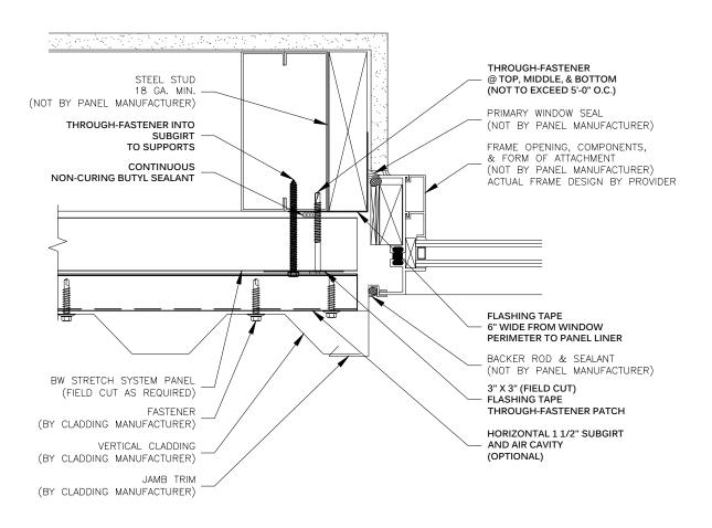
VERTICAL PANEL JOINT CLIP JAMB - w/ HORIZONTAL SUBGIRT BW STRETCH SYSTEM<sup>TM</sup> DRAWING NO:
