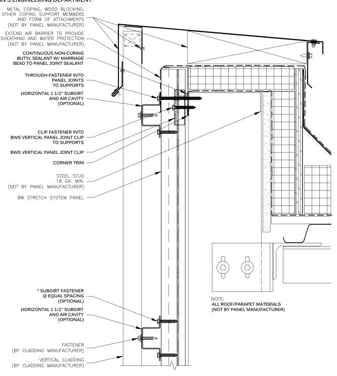
VERTICAL PANEL JOINT CLIP PARAPET - w/ HORIZONTAL SUBGIRT BW STRETCH SYSTEM<sup>TM</sup> DRAWING NO
