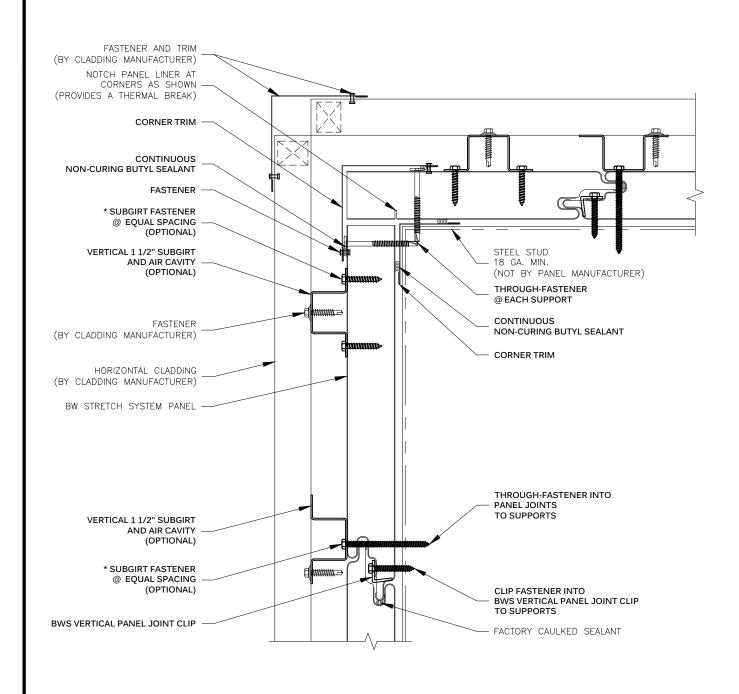
VERTICAL PANEL JOINT CLIP OUTSIDE CORNER - w/ VERTICAL SUBGIRT BW STRETCH SYSTEM<sup>TM</sup> DRAWING NO:
