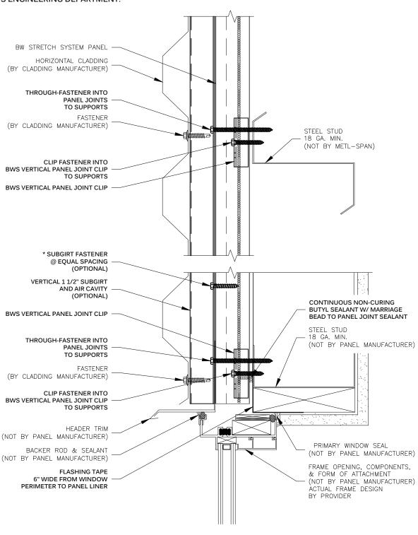
VERTICAL PANEL JOINT CLIP HEADER - w/ VERTICAL SUBGIRT BW STRETCH SYSTEM<sup>TM</sup> DRAWING NO:
