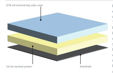
Flurothane® II combines two of the most effective coating technologies in the industry, urethane and fluoropolymer containing 70% Kynar® 500 or Hylar® 5000 resins.
