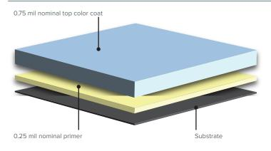
WeatherXL™ is an exceptional silicone polyester coating system which combines the durability of ceramic and other select inorganic pigments with the strength of a breakthrough silicone polyester resin. WeatherXL is known for its remarkable gloss and color retention as well as its superior chalk resistance, which makes it ideal for commercial and industrial buildings.
