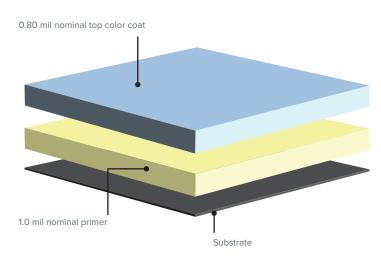
Flurothane® Coastal coatings are a premium fluoropolymer (PVDF) system developed for use in the most extreme coastal environments (less than 1,500' from the coastline). What makes this system unique is the use of an innovative thick film primer.
