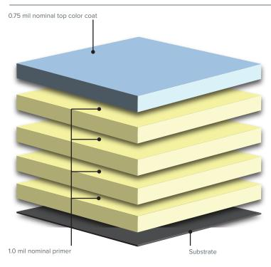
Flurothane® V combines two of the most effective coating technologies in the industry, urethane and fluoropolymer containing 70% Kynar® 500 or Hylar® 5000 resins. Flurothane V is formulated to protect your building project in extremely harsh environments where ultimate protection against salt spray and chemical corrosion is needed.
