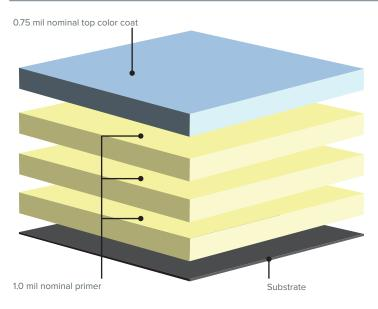
Flurothane® IV combines two of the most effective coating technologies in the industry, urethane and fluoropolymer containing 70% Kynar® 500 or Hylar® 5000 resins.
