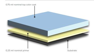
Fluropon® is a premium fluoropolymer coating containing 70% Kynar® 500 or Hylar® 5000 proprietary resins. Fluropon is a field-proven, high performance exterior quality finish for architectural use. It provides outstanding resistance to ultraviolet radiation resulting in exceptional color retention, resistance to chalking and chemical degradation.
