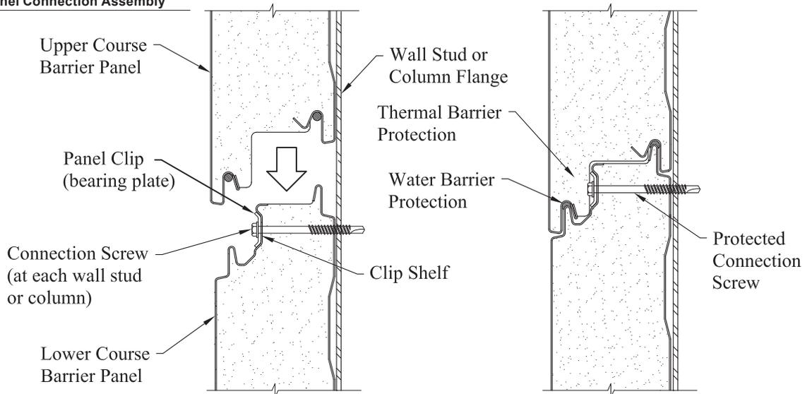
At perimeter conditions, such as base, eave and openings, the panel edges are connected to the framing members with through-panel screws.
