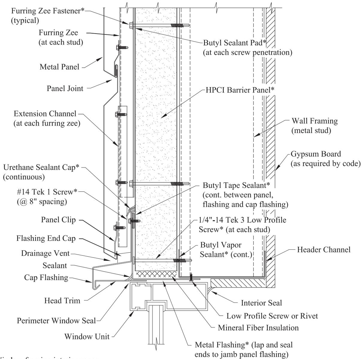
Window framing interior vapor barrier, as required (not shown)
