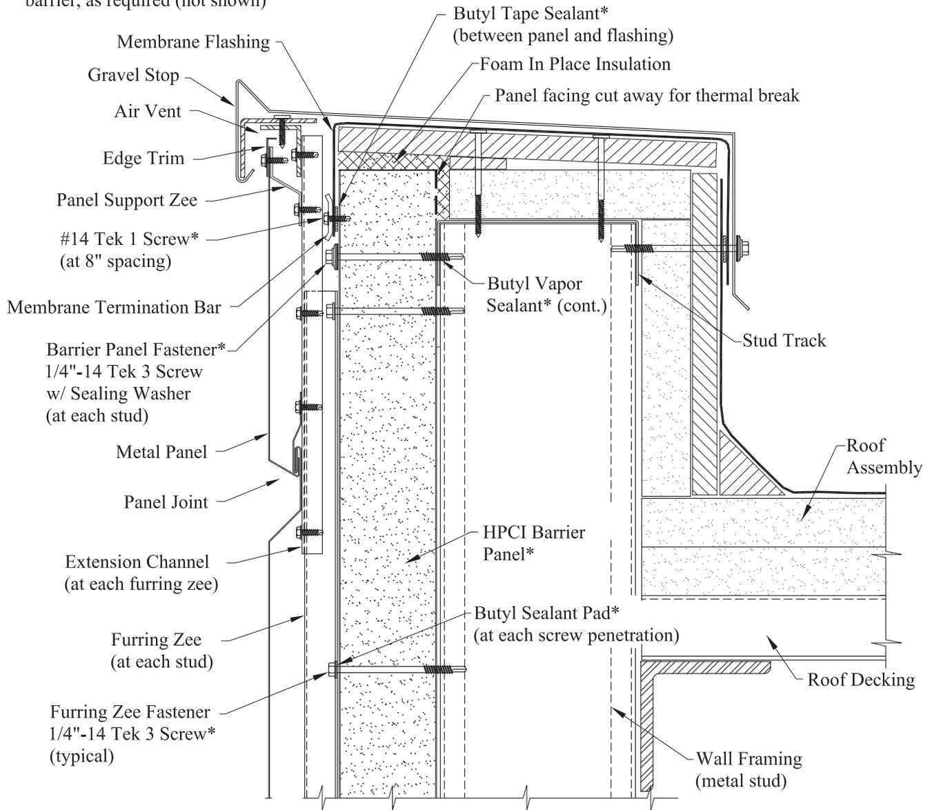
Wall Section At Parapet
