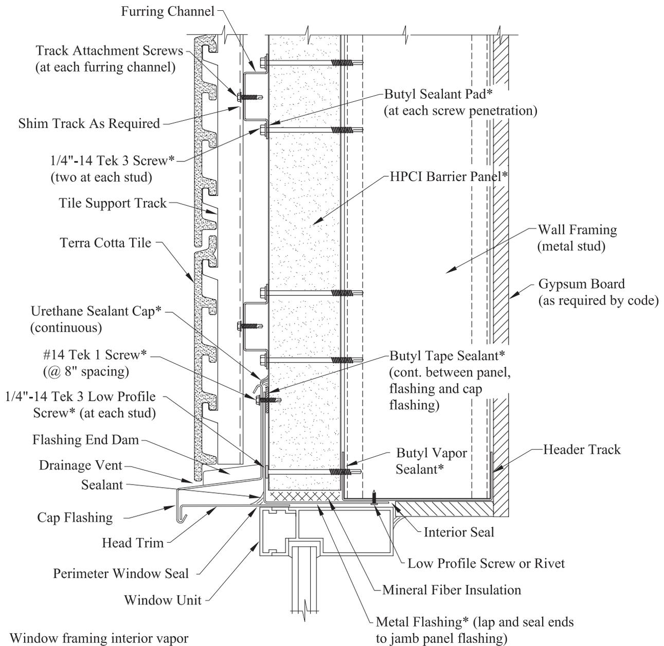
Window framing interior vapor seal as required (not shown)
