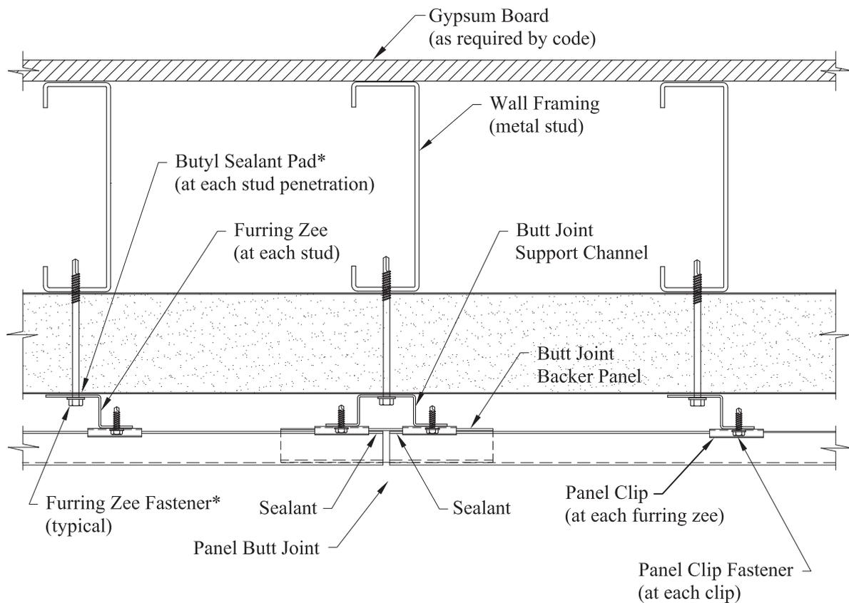
Wall Plan @ Panel Butt Joint
