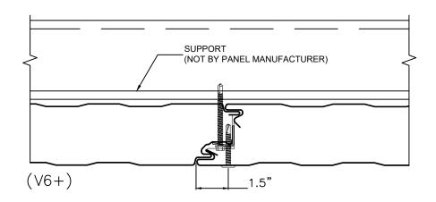
ONE V6 X-SPAN CLIP AT EACH SUPPORT WITH ONE FACE-TO-CLIP FASTENER AT EACH END SUPPORT
