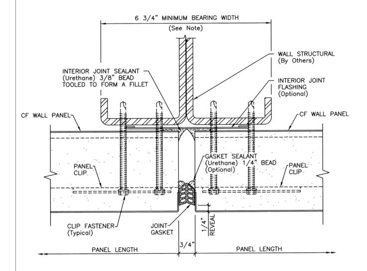
NOTE: Bearing width of wall structural may be reduced to 5 3/4" if load/span design allows connection reduction of one fastener per clip.
