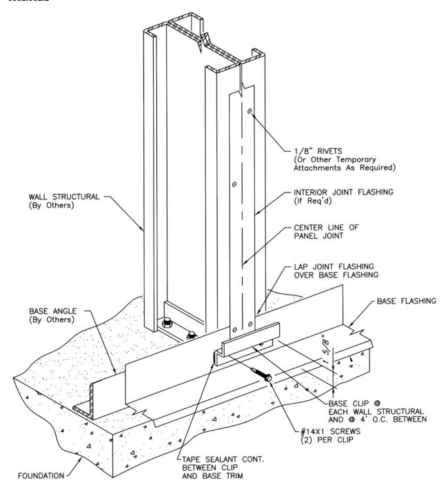
NOTES: 1. It is most important that the base flashing and alignment of the base clips are straight and level. Use a string line or laser to align the base clips at +/- 1/16".
