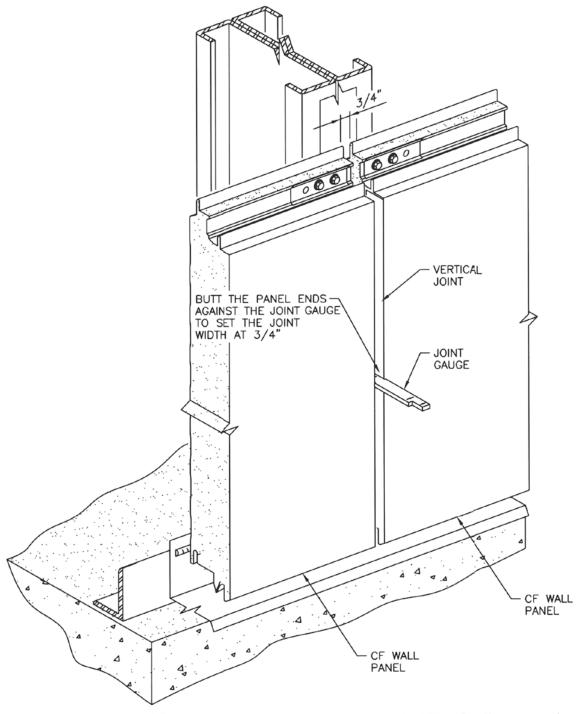
NOTES: 1. Use the 3/4" wide end of the gauge to set the joint width. Set the gauge at mid-point between the horizontal panel joints.
