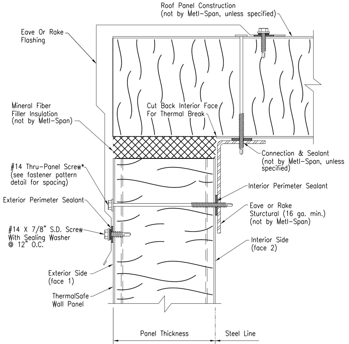
Vertical Panel-Eave Or Rake Detail
