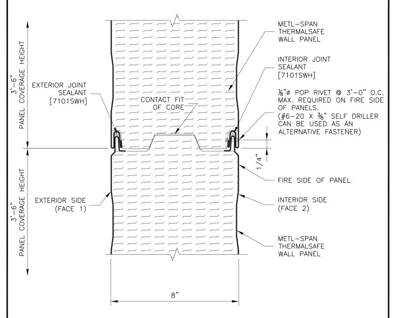
NOTES: 1. IF JOINT SEALANTS ARE REQUIRED, THEY ARE SPECIFIED AS A SILICONE SEALANT IN ORDER TO CONFORM TO THE PANEL'S ASTM E-119 FIRE RESISTANCE RATING.
